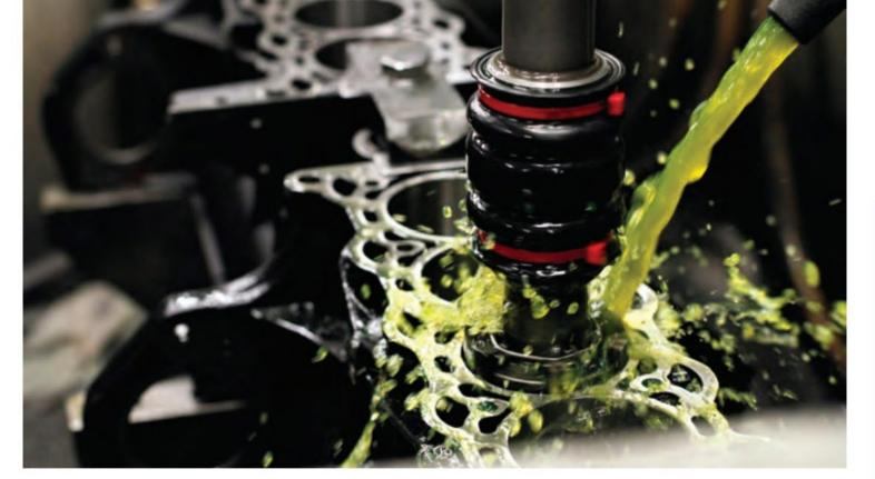
a specific standard for it to be described as such under BSI AU 257:2002. This is a British Standard Automobile Series Code of Practice that applies to the remanufacturing of ICEs. The standard fully details the procedures and operations for the remanufacturing of both spark (petrol) and compression ignition (diesel) engines.
